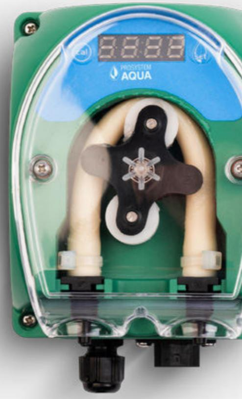
The advanced **ProsystemAqua nutrient automatic controller** is designed for continuous measurement of Ec and dosing of fertilizers or boosters in water tanks, with a flow rate of **0.5 L/hour**.
