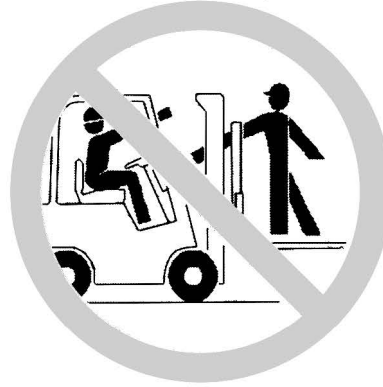
No reach through mast
