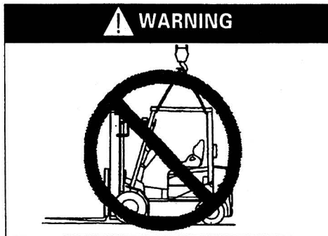
Hoisting with overhead guard prohibite!
